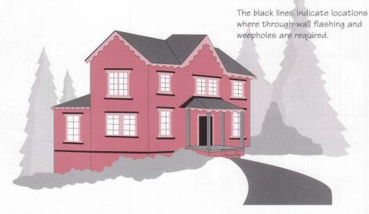
**Note:** Although brick veneer, wood frame construction has proven to be the most durable form of protecting a house from weather, wind-driven rain can penetrate the best brickwork. Southern Brick Institute strongly recommends compliance with the flashing and weephole requirements of the Cabo and Standard Building Codes.
