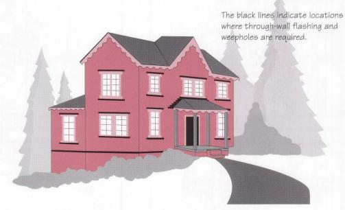
**Note:** Although brick veneer, wood frame construction has proven to be the most durable form of protecting a house from weather, wind-driven rain can penetrate the best brickwork. Southern Brick Institute strongly recommends compliance with the flashing and weephole requirements of the Cabo and Standard Building Codes.
